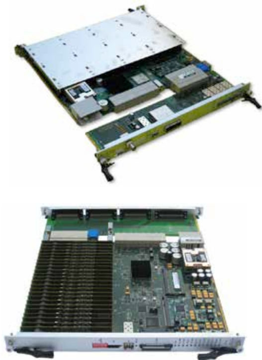
Figure 4: IPFN ATCA PCIe switch card and RTM_host (top) and Prototype of the ATCA PCIe node card for control and data acquisition developed at IPFN.
