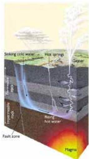
Figure 1 – Conceptual model of a geothermal system. Adapted from Gao (2005) in [8].
