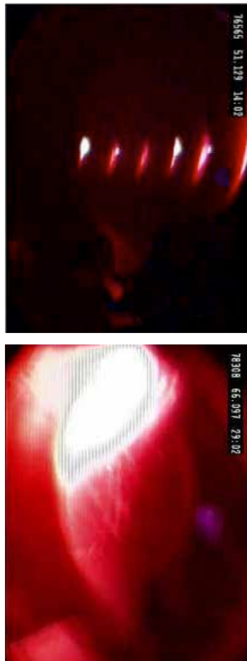
Figure 2: JET interior during a plasma discharge. Top: Plasma before the disruption. Only mild interaction with the side walls is observed; Bottom: Large VDE disruption at JET. Huge thermal loads are observed on the Plasma Facing components on the top of the machine.
