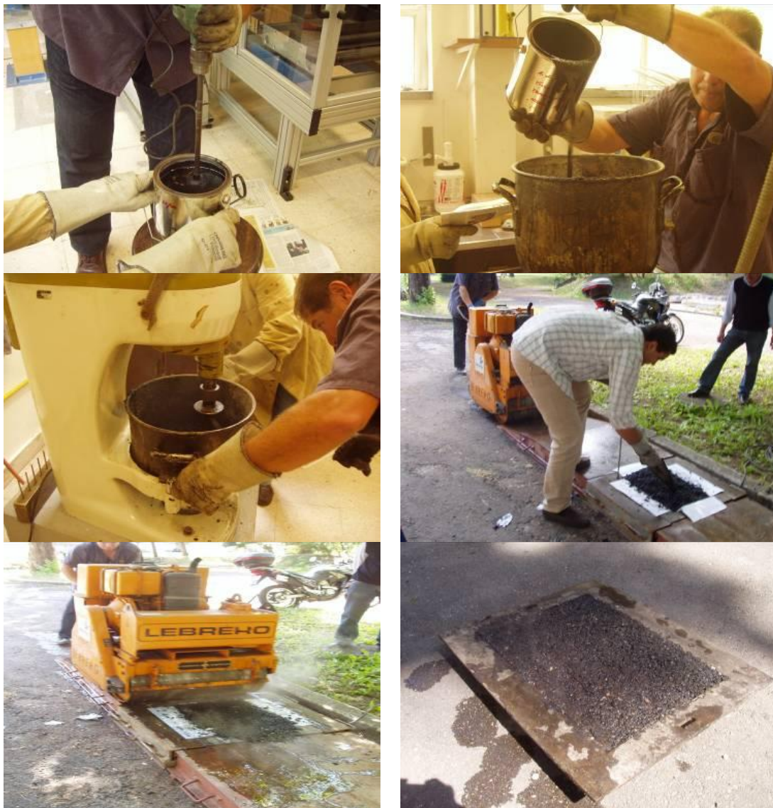
Figure 5 – Laboratory mixtures manufacture phases (ARO-granite-lab and ARG-gravel-lab)
