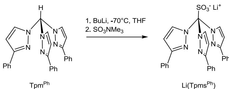
Scheme 1 – Synthesis of tris(3-phenylpyrazolyl)methanesulfonate species as the lithium salt, \text{Li}(\text{Tpms}^{\text{Ph}}) [7].
