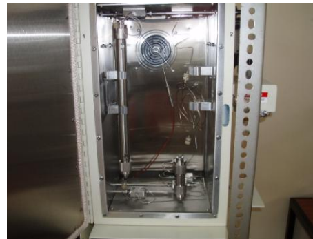
Figure 3 – Extraction vessels inside of the furnace (heating system).
