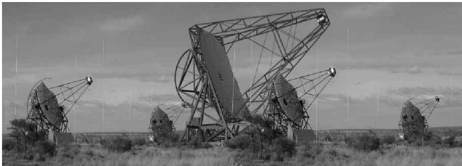
Fig. 1. Photo of the current four-telescope H·E·S·S· Phase-I array, with an artist’s impression of the Phase-II 30m \varnothing telescope in the centre of the array superimposed.
