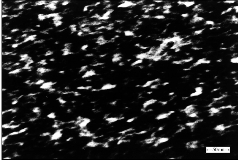
Figure 2. Dark-field transmission electron micrographs of a hemoilmenite crystal (weakly magnetic region) taken with the ordering reflection g = 0003 and showing tiny cation-ordered domains (typically 20-40nm) in a cation-disordered matrix. Ordered domains tend to be flattened along the direction of the basal hexagonal plane.
