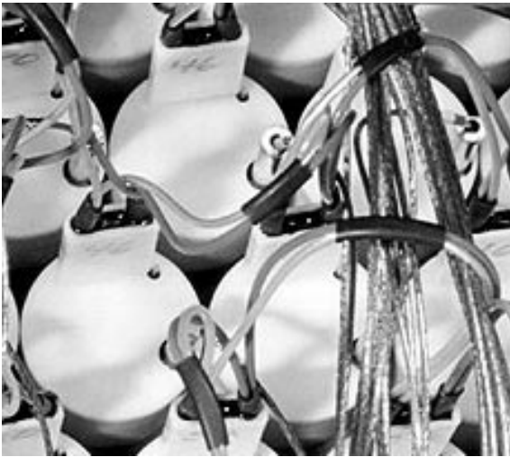
Figure 37. Photograph of a group of DIRC PMT bases with signal and HV cables attached.
