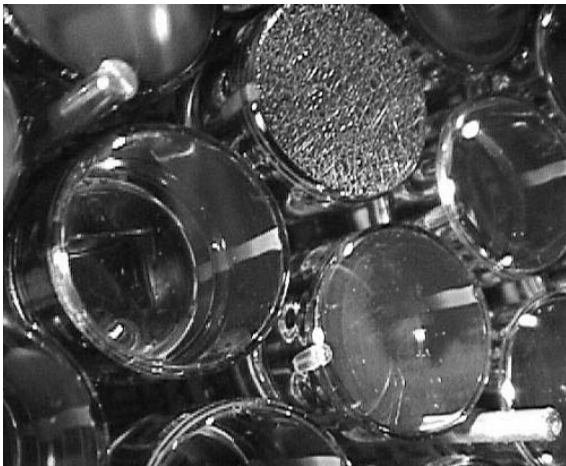
Figure 36. Example of an undamaged PMT (left), a “frosty” PMT (top), and a “milky” PMT (bottom), observed in the drained SOB roughly one year after it was first filled with ultra-pure water.
