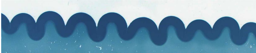
Figure 3: Side view of the gel top layer (colored with ink) after swelling. Thickness h = 3 mm (after swelling), wavelength \lambda = 8.9 mm and amplitude A = 5.1 mm.
