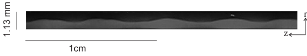
Figure 16: Interface profile in a plane (r, z) for a sample of CPCl/NaSal (6.3%) in 0.5 M NaCl brine at T=21.5^\circ\text{C} . The mean shear rate is \dot{\gamma} = 9\text{s}^{-1} and the snapshot is taken after the steady banded state is achieved.
