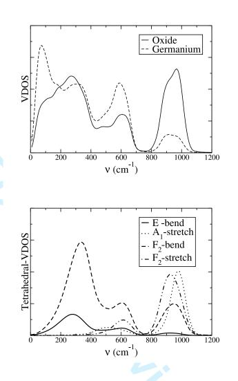
FIG. 7: The vibrational densities of states, for the DIPPIM, of both type of ions (top panel), and their projections in terms of the A (symmetric stretch),  $F_2$  (asymmetric stretch), E (bend), and  $F_2$  (bend) modes of the Ge0<sub>4</sub> tetrahedra (bottom panel).
