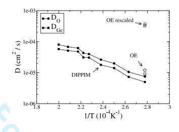
FIG. 4: Diffusion coefficients obtained with a DIPPIM potential at different temperatures; data points obtained with both the original and rescaled OE potentials at 3600 K are also presented.
