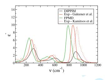
FIG. 5: Imaginary part of the dielectric function, calculated for simulations carried out with the DIPPIM potential, compared to FPMD simulation<sup>10</sup> and experimental results<sup>2,3</sup>.
