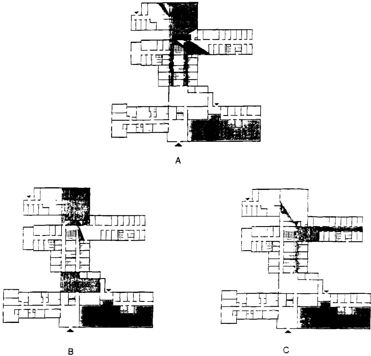
FIGURE 9.8: Isovists of MAR Showing Views from (a) the Control Room, (b) the Multipurpose/Dining Space and Activity Room (in Two Separate Isovists), and (c) the Boys Dayroom
