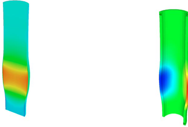
FIGURE 2. Solution of the 3-d model at time t = 50E - 4 for a Young modulus E_1 = 4E6 . Left: fluid velocity along the z axis. Right: displacement of the structure along y axis.
