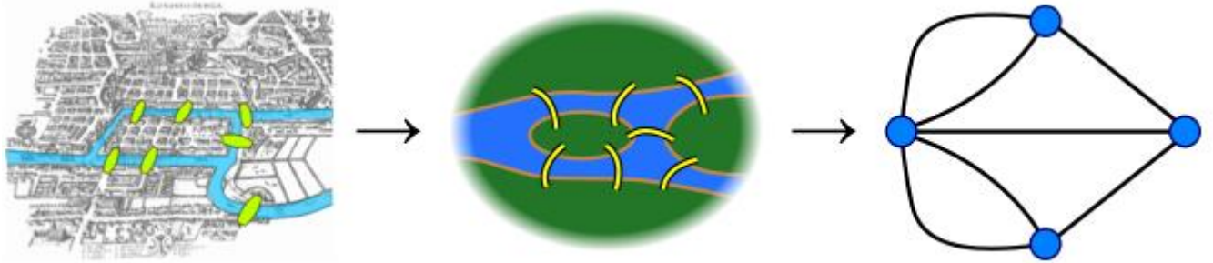
Figure 1.3: The map of Königsberg (left), a diagram to emphasize the structure of the river (middle) and the abstraction of the topology of this structure as a graph (right). From Wikipédia.
