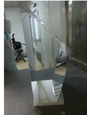
Figure 4: Finished FBLOCK, made of solid Corning 7980 fused silica.
