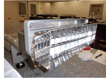
Figure 3: New wedge glued to the bar box window.
