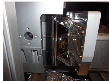
Figure 5: Details of coupling between FBLOCK, new wedge and bar box. A gap between FBLOCK and new wedge is filled with the RTV.
