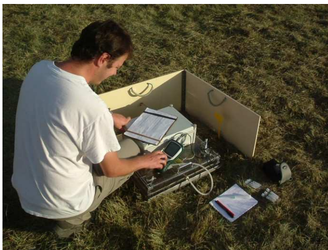
Figure 3: Gas flux measurement on a volcanic site. Isotopic samples are collected with a syringe and stored in Exetainer vials.
