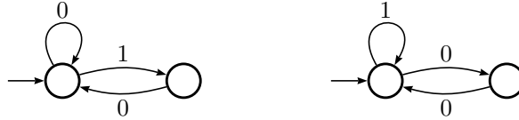
Fig. 4: Finite automata for the G -shift (left) and for the (-G) -shift (right)
