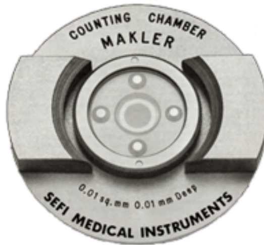
Fig. 1 Makler counting chamber, metallic base tool to evaluate sperm amount. (Makler, 1980)
