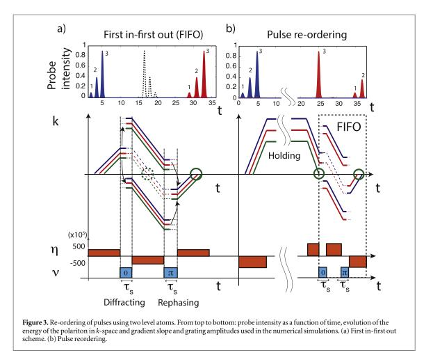
a similar FIFO read-out as in the A-GEM: the pulses come out without time-reversal but now using only twolevel atoms and this purely dispersive diffraction control.
