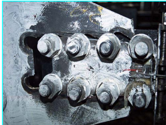
(a) The force distribution in T-stub member (b) The typical block shear failure of T-stub member
