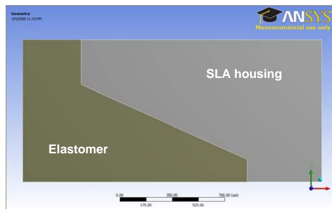
Figure 5.2 2-D geometry model of a SHA chamber filled with PDMS
