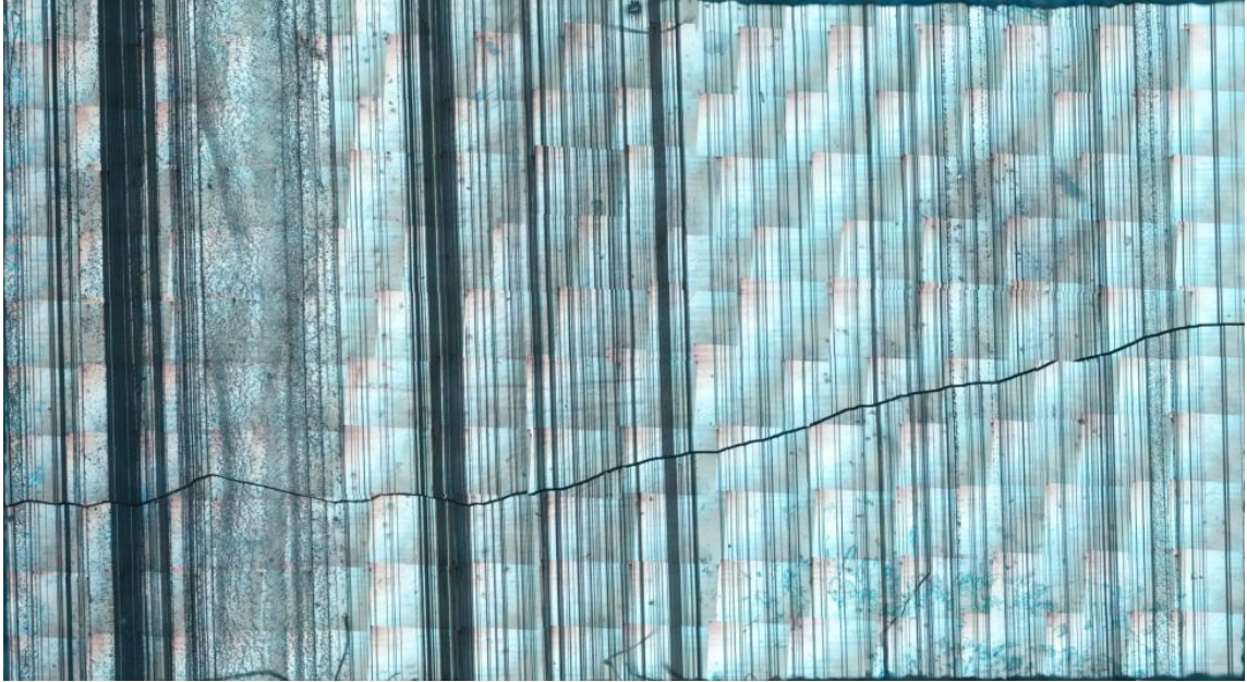
Figure 18: EFG Area 1 (D1-3). Wafer was cracked during measuring. Area Size: 14mm x 8mm.
