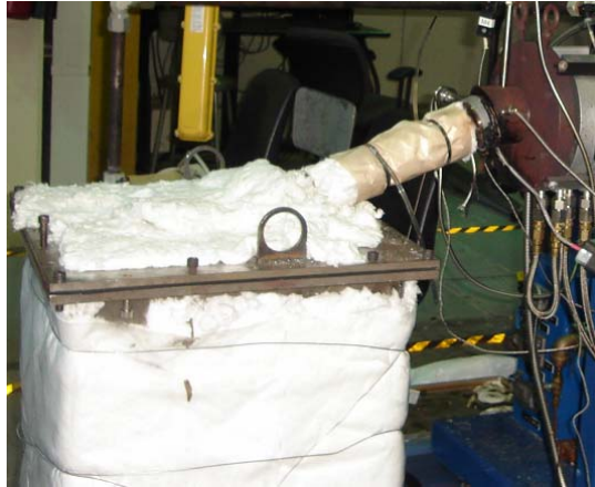
Figure 6.19: Picture of die attachment for collection of residual product
