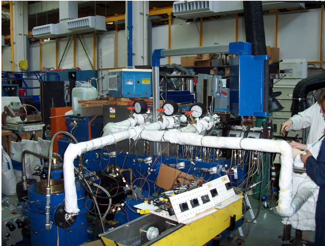
Figure 6.18: Picture of extruder with vacuum system attachment 1
