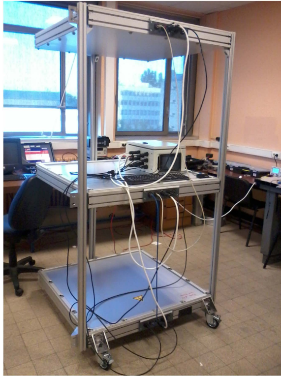
Figure 8. Picture of the muon telescope used for the SHADOW experiment, here during the open-sky calibration phase. The three detection matrices are horizontal. The calibration gives access to the effective acceptance. The control box embedding a mini-PC, a common clock distribution system, a network switch is visible on the middle matrix.
