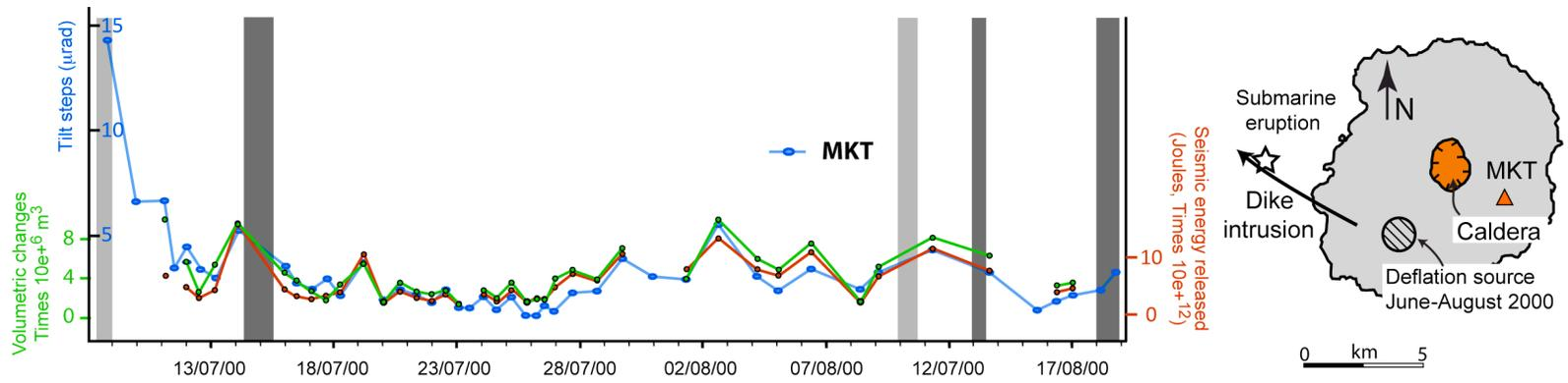
**Figure 4.** Evolution of the tilt step amplitude recorded at the MKT station [after Yamamoto *et al.*, 2001] and of the volumetric changes [after Kumagai *et al.*, 2001] and the seismic energy released inferred from the 39 VLP events [after Kikuchi *et al.*, 2001] during the caldera collapse of Miyakejima.
