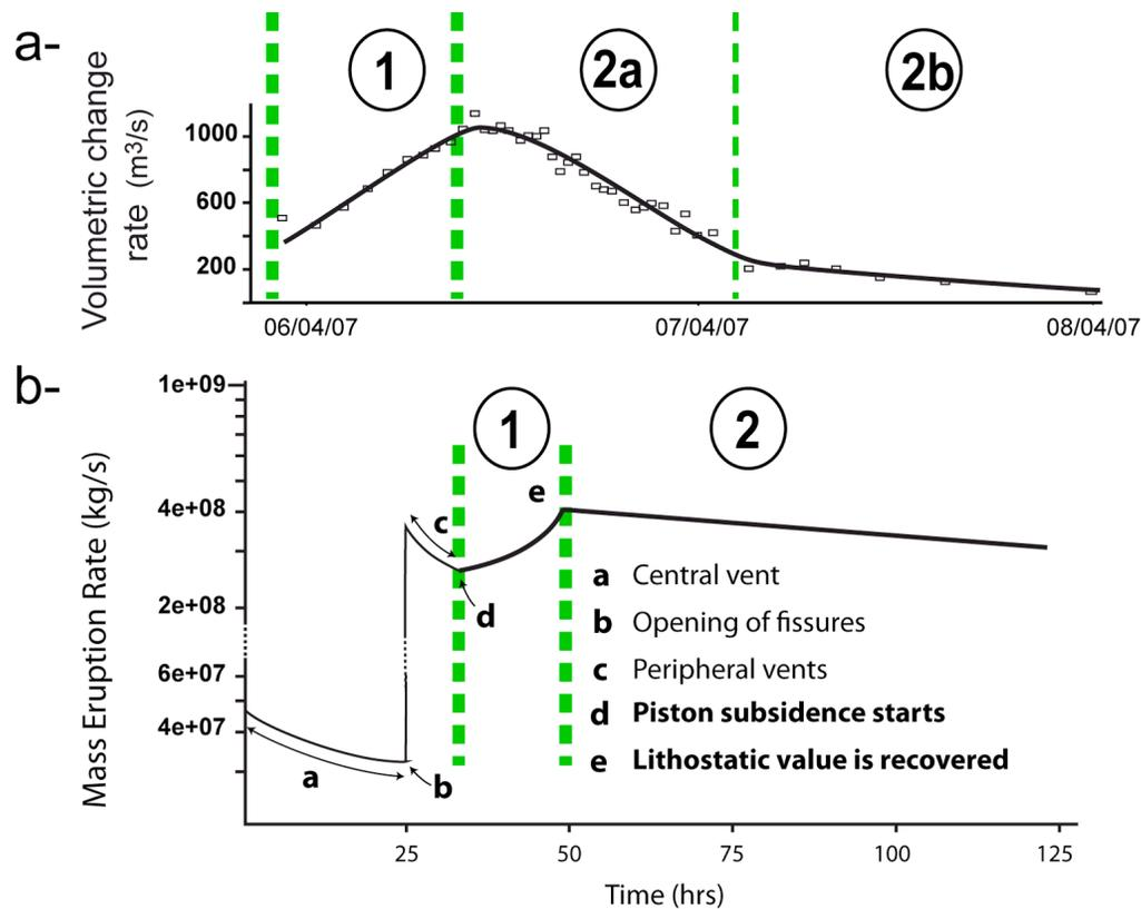
**Figure 8.** Twofold collapse dynamics for (a) basaltic and (b) silicic calderas. Figure 8a gives the rate of magma outflow determined for the caldera collapse of Piton de la Fournaise, while Figure 8b gives the mass eruption rate calculated by *Folch and Martí* [2009] for silicic calderas.
