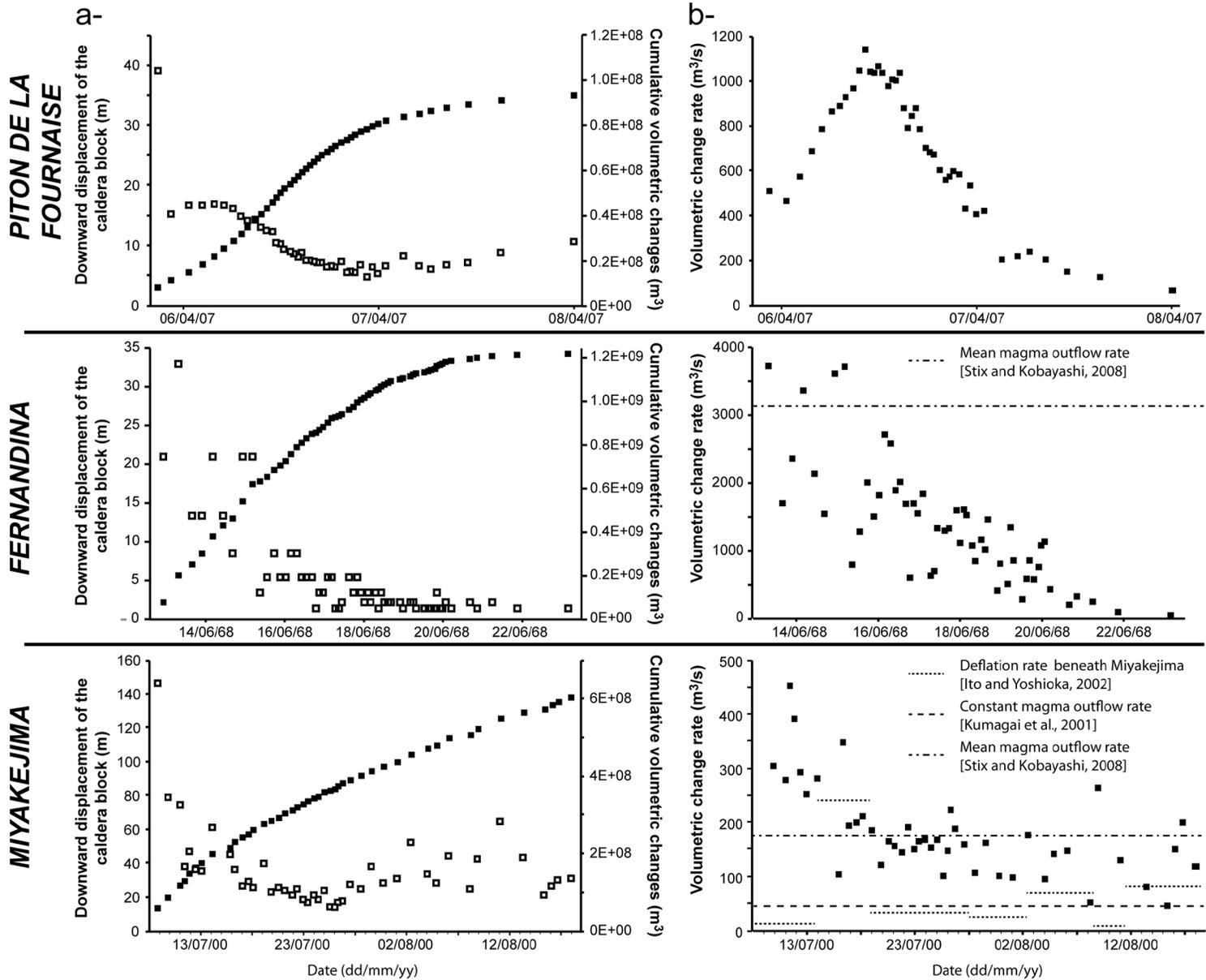
**Figure 3.** (a) Downward displacements during each collapse increments and the resulting cumulative volumetric changes in the magma chamber. (b) Volumetric change rates inferred from the volumetric changes and the time interval between two collapse increments. See text for explanation.
