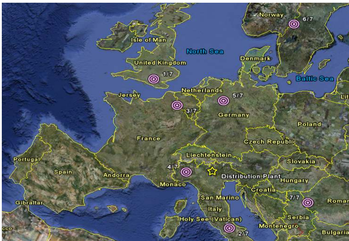
Figure 45 Geographical location of centres of gravity for a seven cluster analysis using GK algorithm with database 3. (Source: Author; Google Maps)
