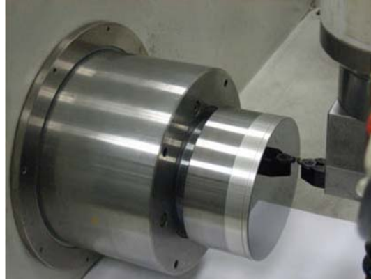
Figure 3.13 End turning set-up on the ultraprecision machine tool
