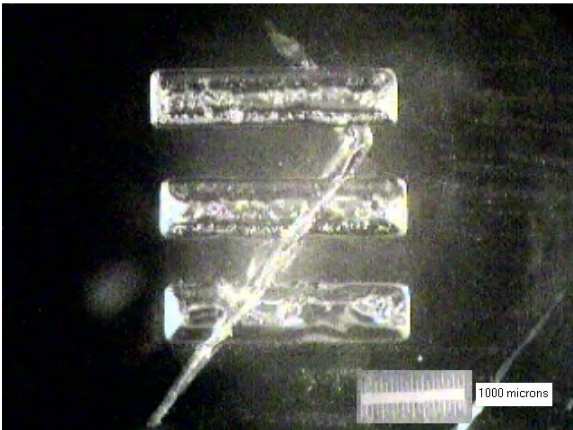
Figure 5.14 Rectangular layers cured by imaging bitmap in Figure 5.13 onto the resin surface
