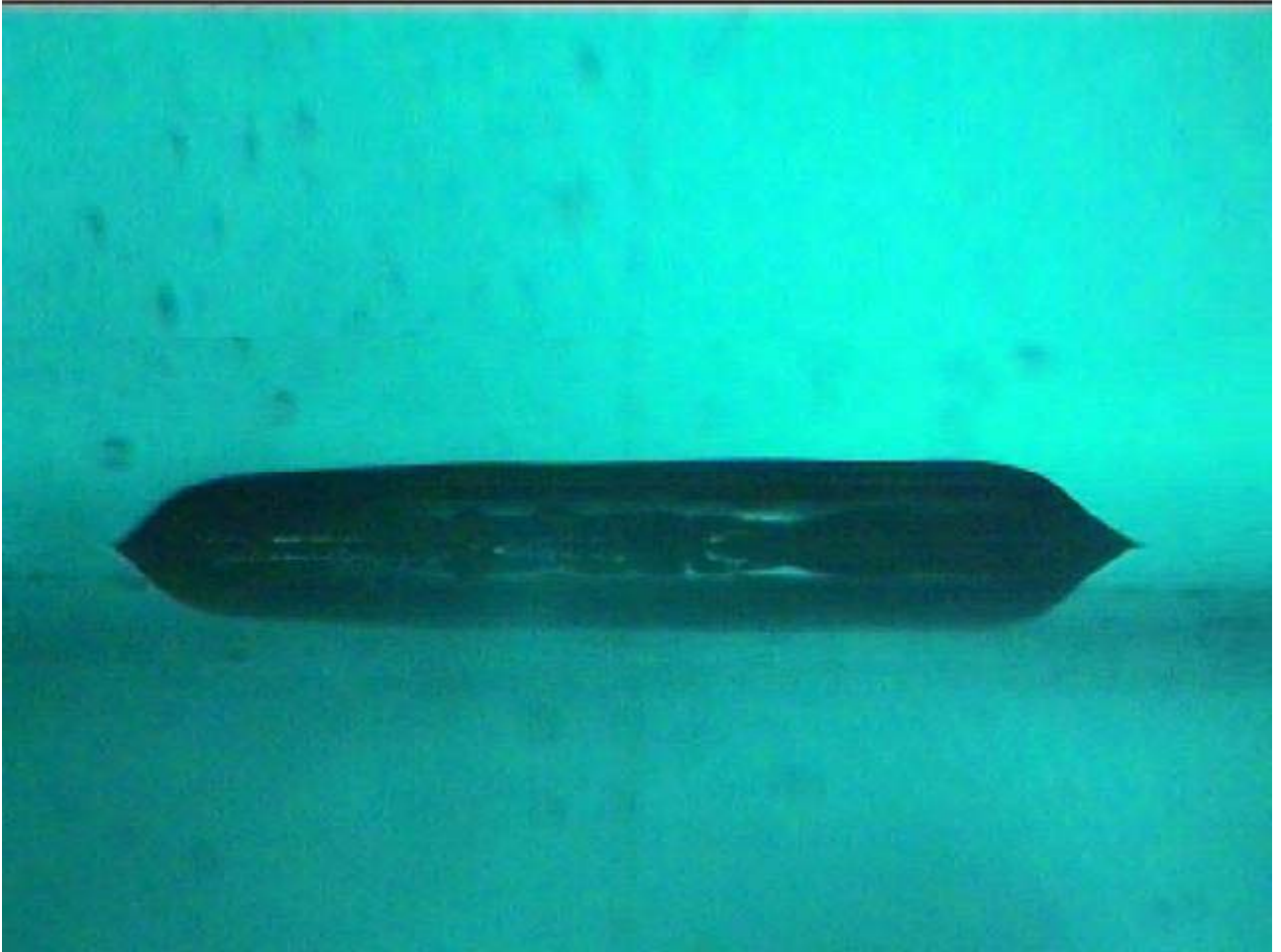
Figure D. 9 Layer cured for 30s exposure: Validation layer 3
