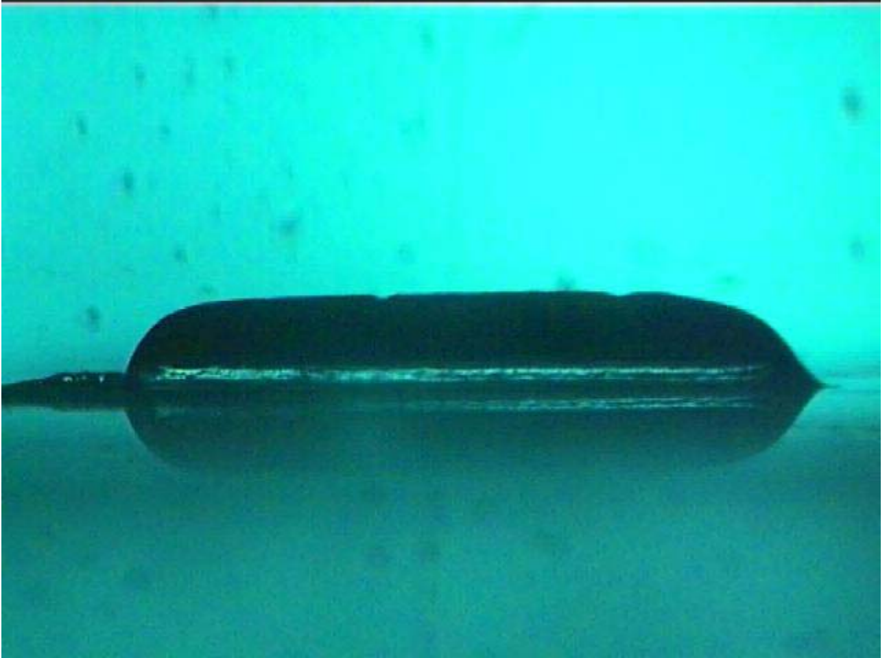
Figure E.7 Waiting time between exposures = 60s. Test layer 2
