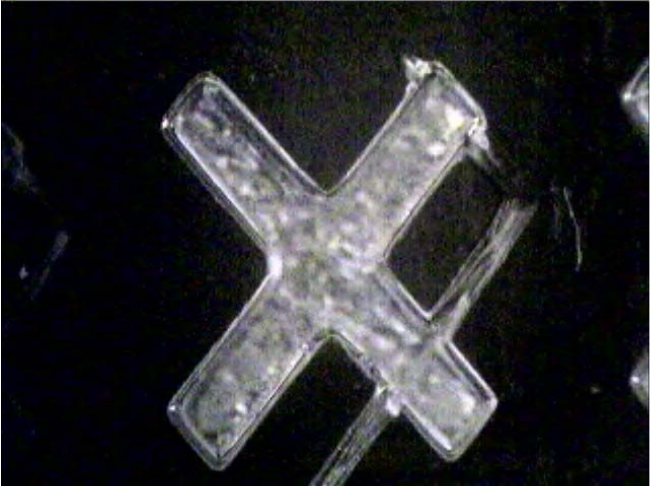
Figure A. 8 Calibration scale for measuring the dimensions of the test layers
