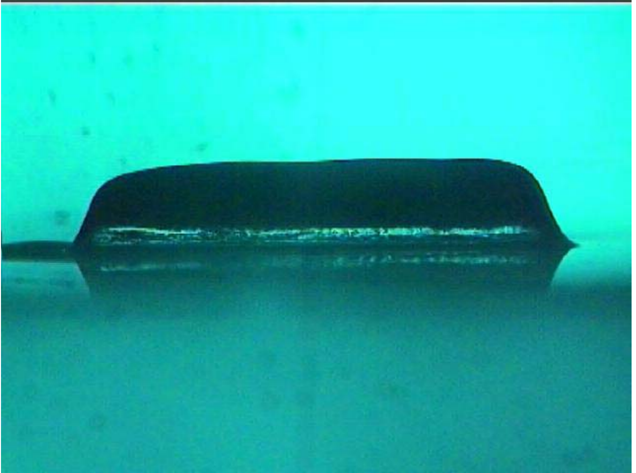
Figure D. 17 Layer cured for 45s exposure: Validation layer 2
