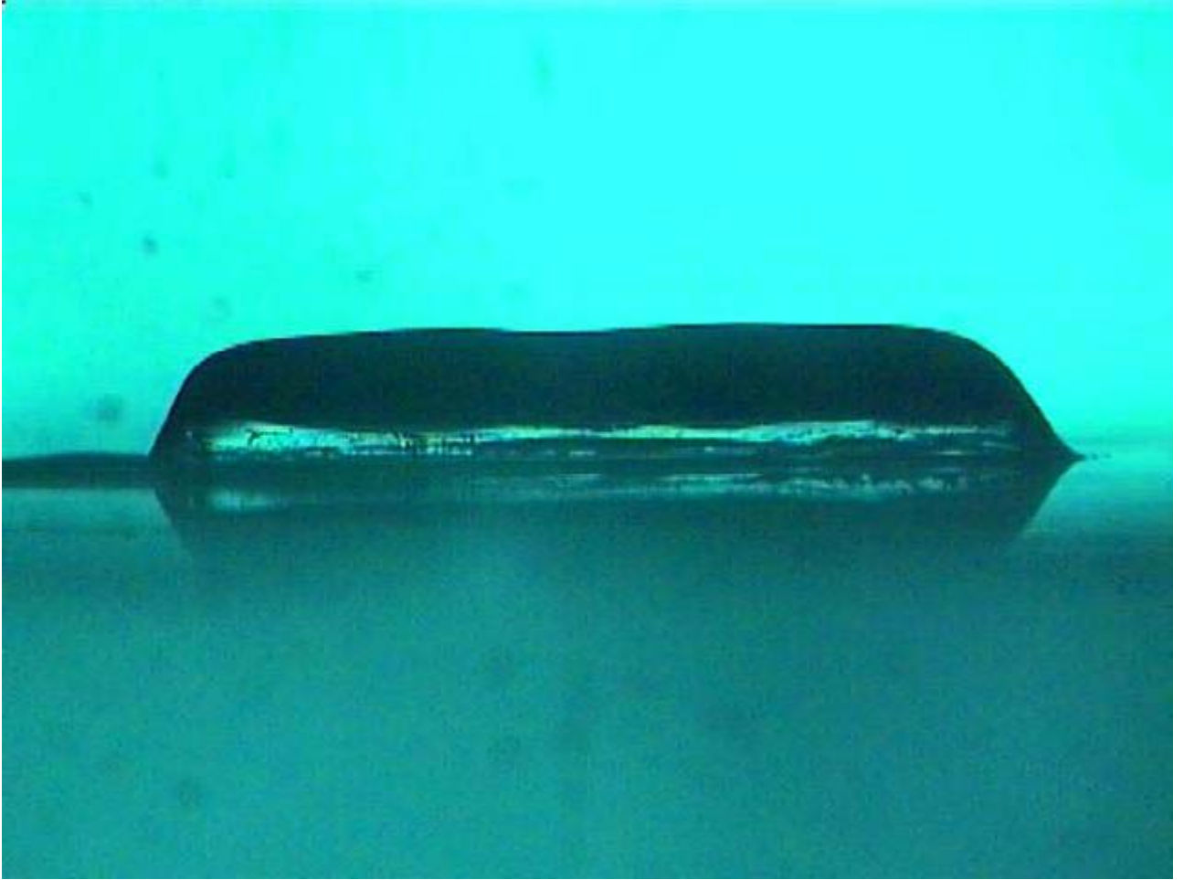
Figure D. 13 Layer cured for 40s exposure: Validation layer 1
