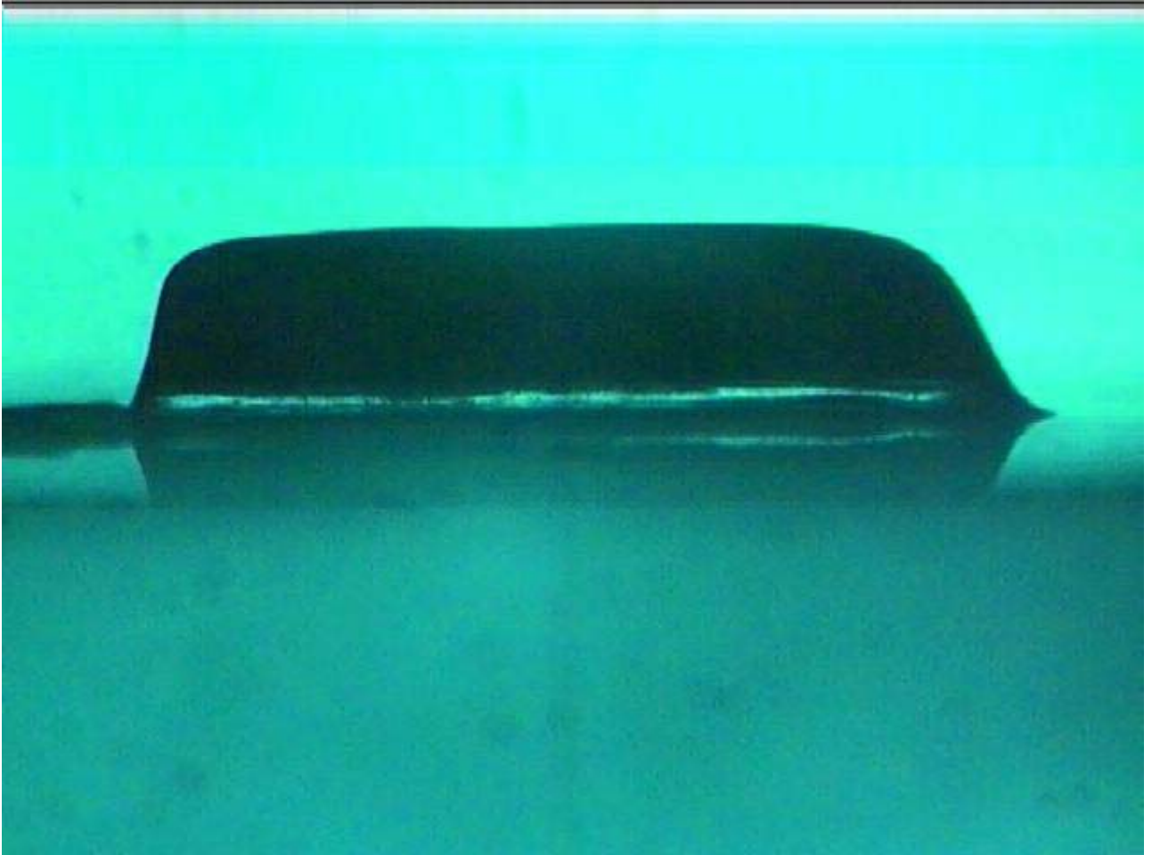
Figure E.2 Waiting time between exposures = 4s. Test layer 2
