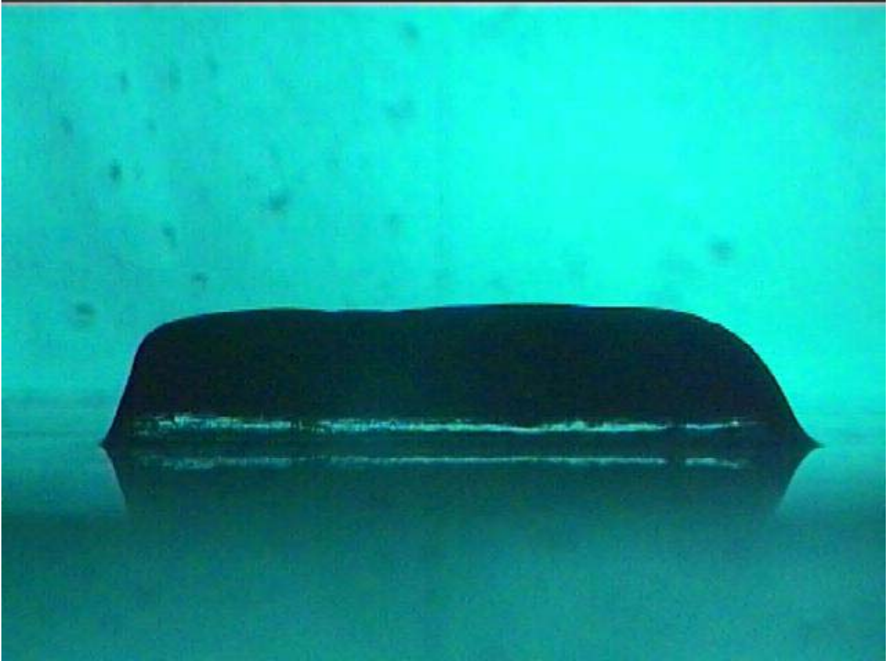
Figure D. 20 Layer cured for 50s exposure: Validation layer 2
