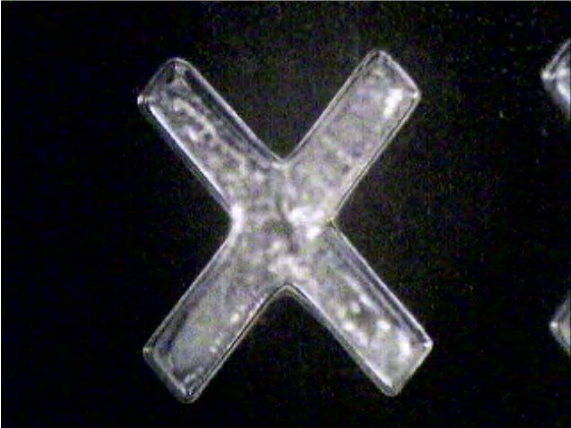
Figure 5.8 Layer cured by imaging the bitmap in Figure 5.6 onto the resin surface
