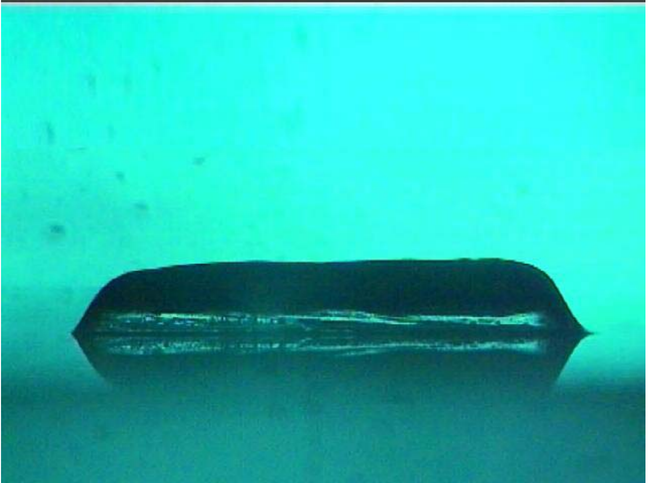
Figure D. 15 Layer cured for 40s exposure: Validation layer 3
