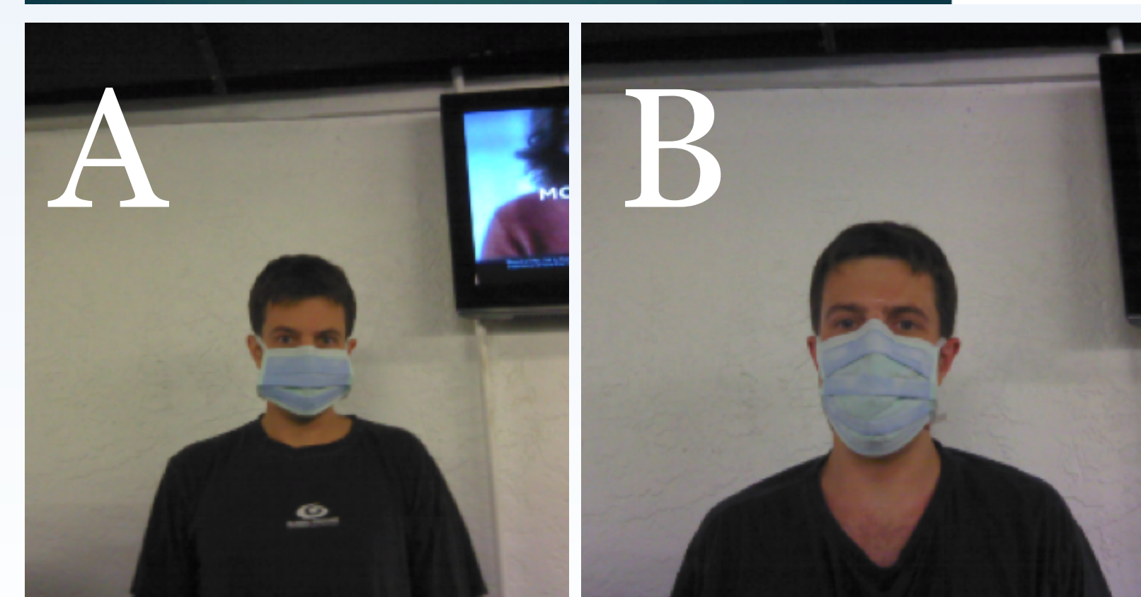
Figure 3 A) The 89°F mask before the wearer runs is a dark blue color and B) post-run the 89°F mask fades in color overall with clear/white areas forming between the flaps and around the chin and nose.
