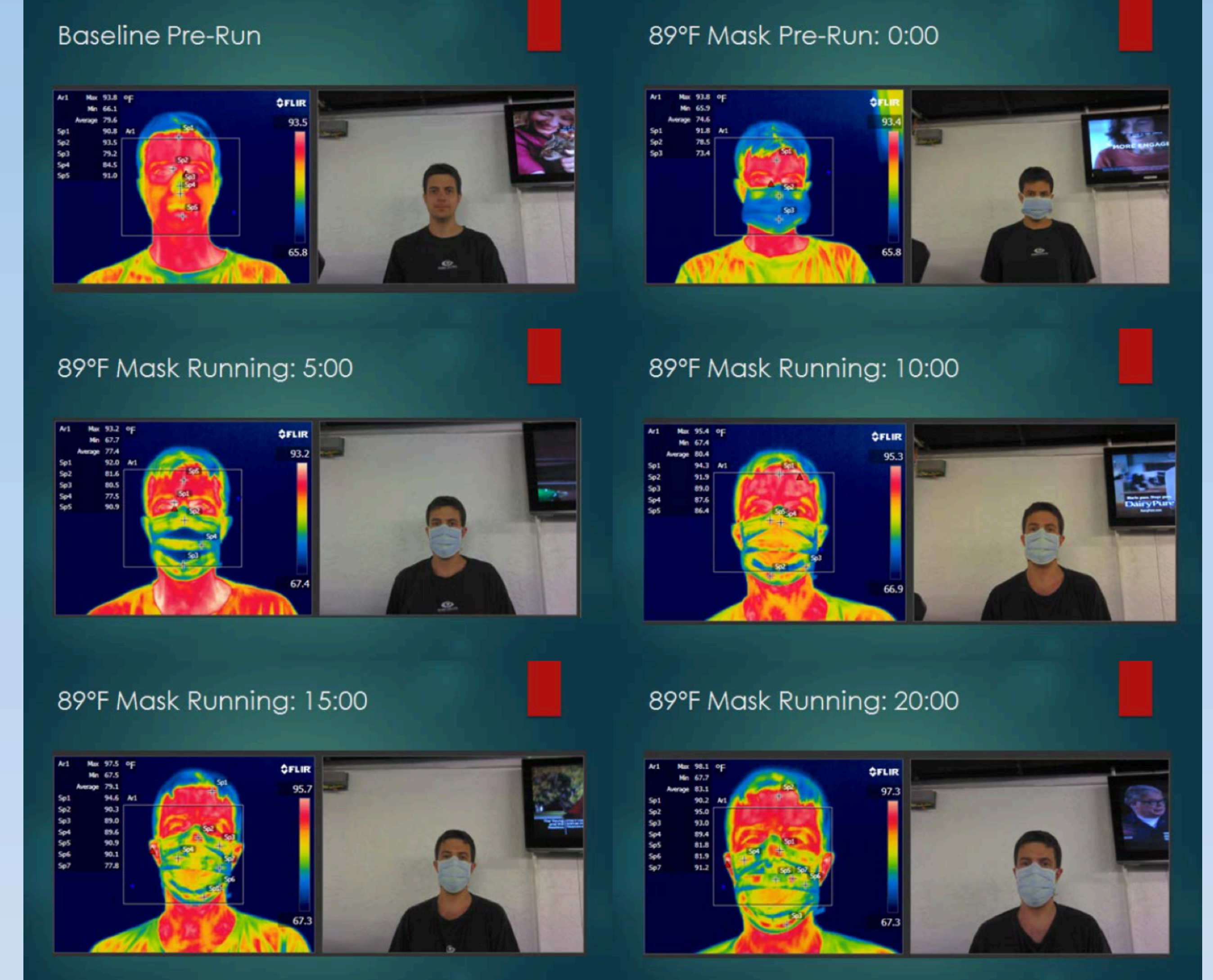
Figure 4: Temperature sensitive mask created with 89°F dye worn while running, showing increasing color change from blue to white in response to increasing skin temperature. An increase in mask temperature using the thermal camera was also apparent.
