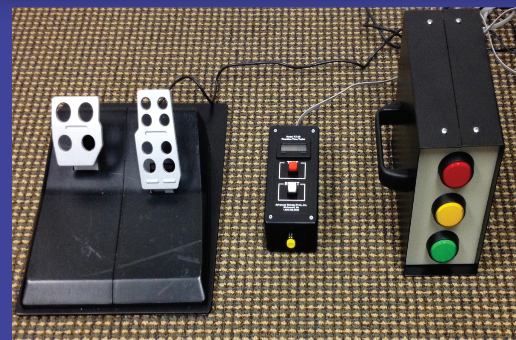
Figure 1: Brake Reaction Test (BRT) device for measuring brake time after a stimulus.
