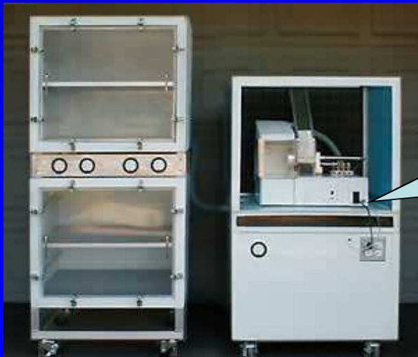
Collecting and mixing chamber for rodent exposure studies
