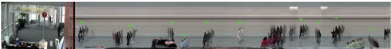
Fig 9. Temporal profile of a video recording an indoor environment with three sampling lines (red). The transparency of slices increases from right to left. The arrows on top of targets show their passing in leftward or rightward direction.
