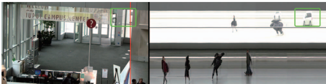
Fig. 5 A temporal slice captures a passing car in its complete shape (right), which is unnoticeable as a complete shape in the video frame (left). The red line is sampled for the temporal slice.
