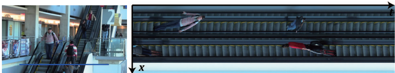
Fig. 6 A horizontal line samples apparent vertical motion to obtain a temporal slice. The targets are skewed due to slanted motion vector with respect to the sampling line (blue). The high image quality allows capturing details.
