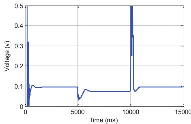
Figure 6. Controller command to the proportional valve in regulation under low wind speed disturbances.
