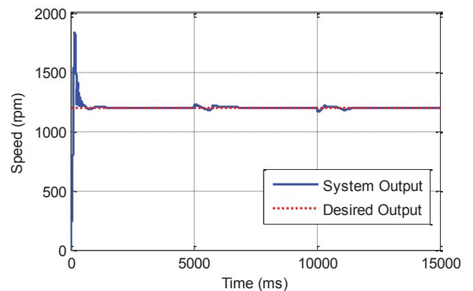
Figure 8. Regulation response of the system under high wind speed disturbances.
