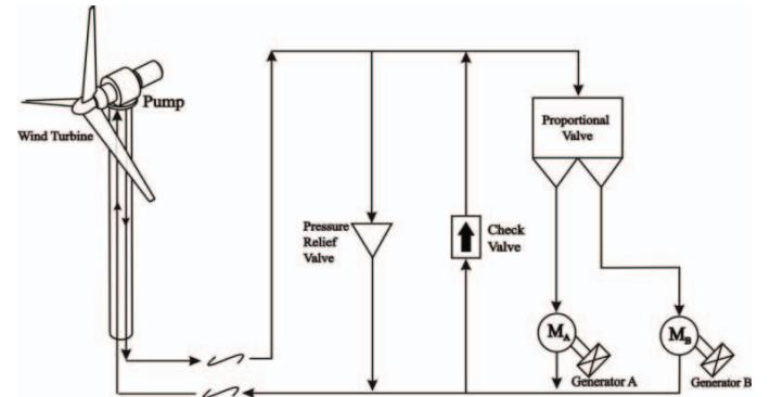
Figure 1. Schematic of hydraulic wind power transfer systems.
