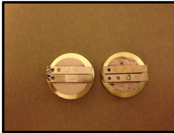
FIGURE 14. A) Sputter-coater (Denton Vacuum Desk II) and B) Zirconia bars sputter-coated with gold prior to SEM imaging.
