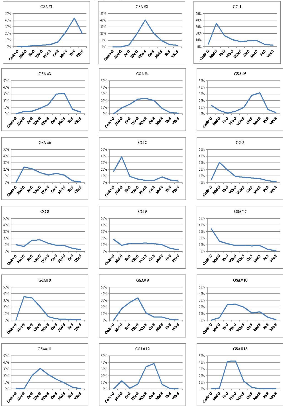
Appendix B: Grain size distribution of SC0802 samples (sand and gravel fractions)
