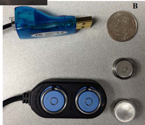
Figure 1. The microcosm experimental setup (A) and a photo of iButtons and iButton data reader (B). The US quarter is for scale.
