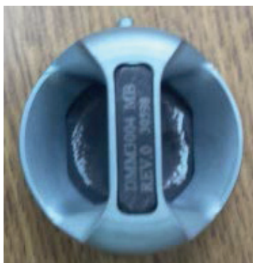
Fig. 15. Image of modular die showing the wear pattern
