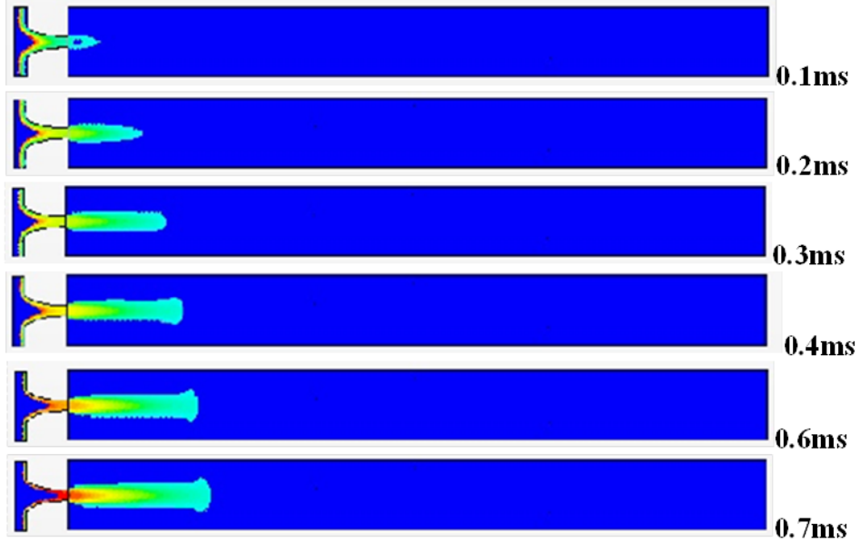
Figure 4.17 Injected Gas for \langle m_{0.2 \leq Y_{HG} \leq 0.8} \rangle above Critical Temperature of 700 K in the Main Chamber
