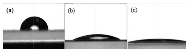
Figure 5. Hydrophilicity test on differently treated PS film. Only PS film in the device has direct surface contact with reactant, thus it is specially treated to acquire different surface property. (a) without treatment, contact angle=92° (b) PS film after oxygen plasma treatment, contact angel= 25° (c) PS film after hydrophilic coating, contact angle=17°
