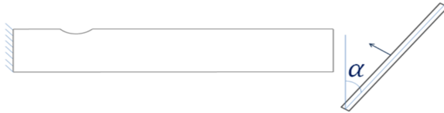
Figure 4-4: Tube with geometric imperfection subjected to an impact at angle \alpha .
