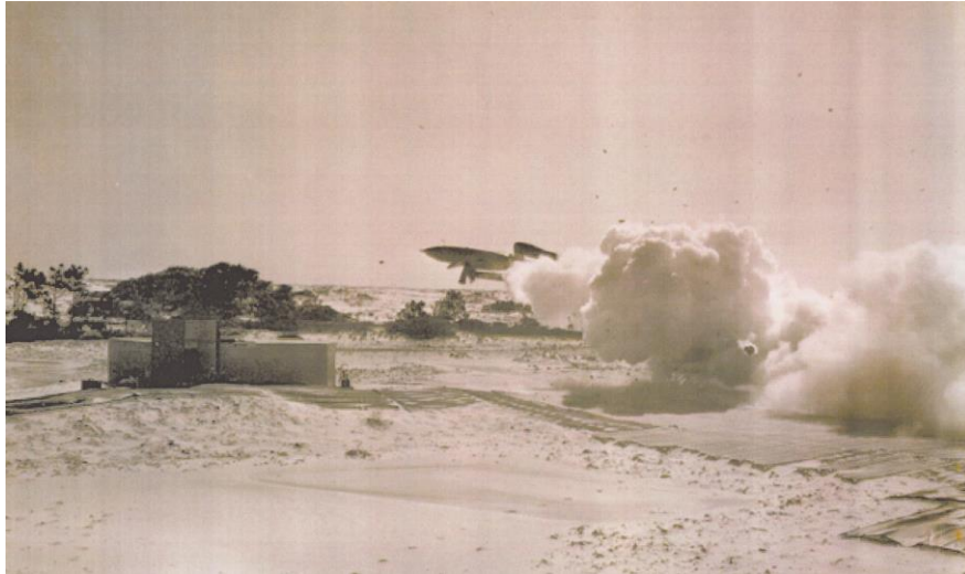
JB-2 departing 80K248, note blockhouse/bunker and launch pad. 165
