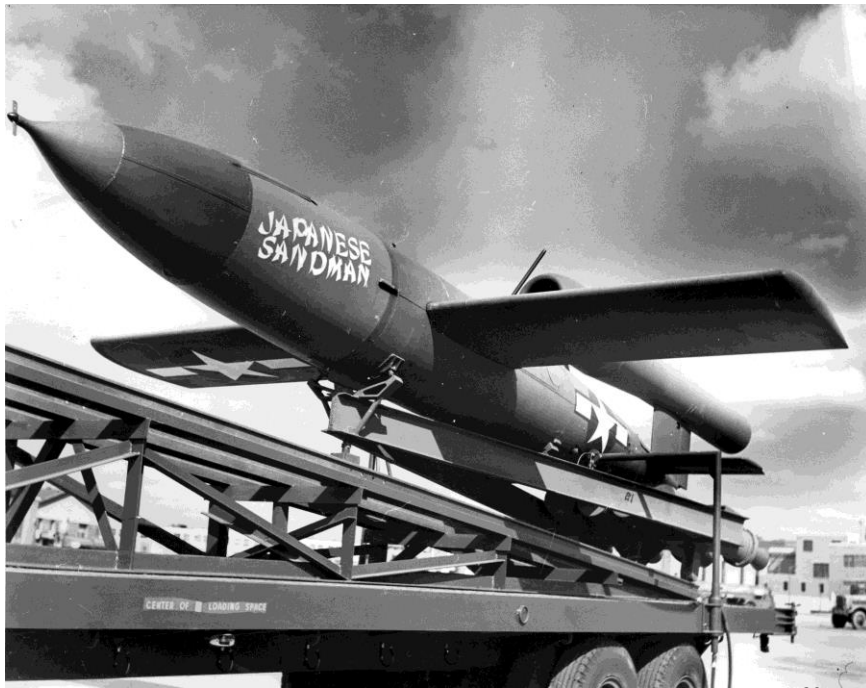
JB-2 on “zero launch” mobile ramp at Range 64, 1945. 80
