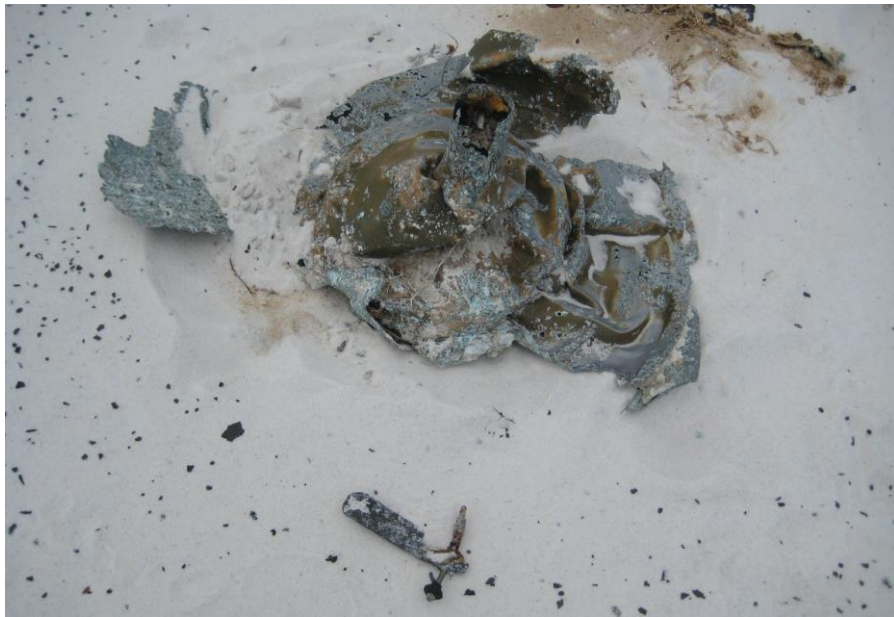
Crushed nose cone and broken impeller/air log from JB-2 on 8Ok246, June 2012. 177
