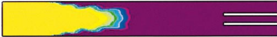
Fig. 12 Fuel ( C_3H_8 ) Concentration in the channel after a long time (10.1 ms). Refer to Fig. 11 for field plot color map.
