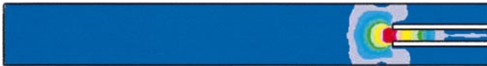
Fig. 8 Mach number distribution of partition exit flow. Hot gas injection. Time=0.165 ms. (Refer to Fig. 7 for color map.)
