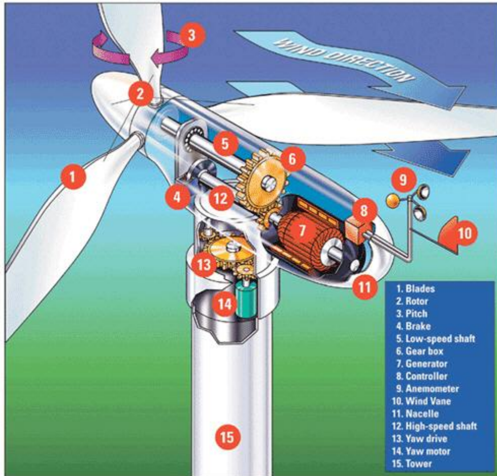
Figure 1.1 Wind Turbine Components [41]
