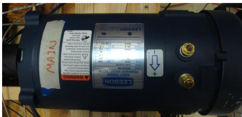
Figure 6.3 DC Motor coupled to the shaft of Pump B and Motor A
