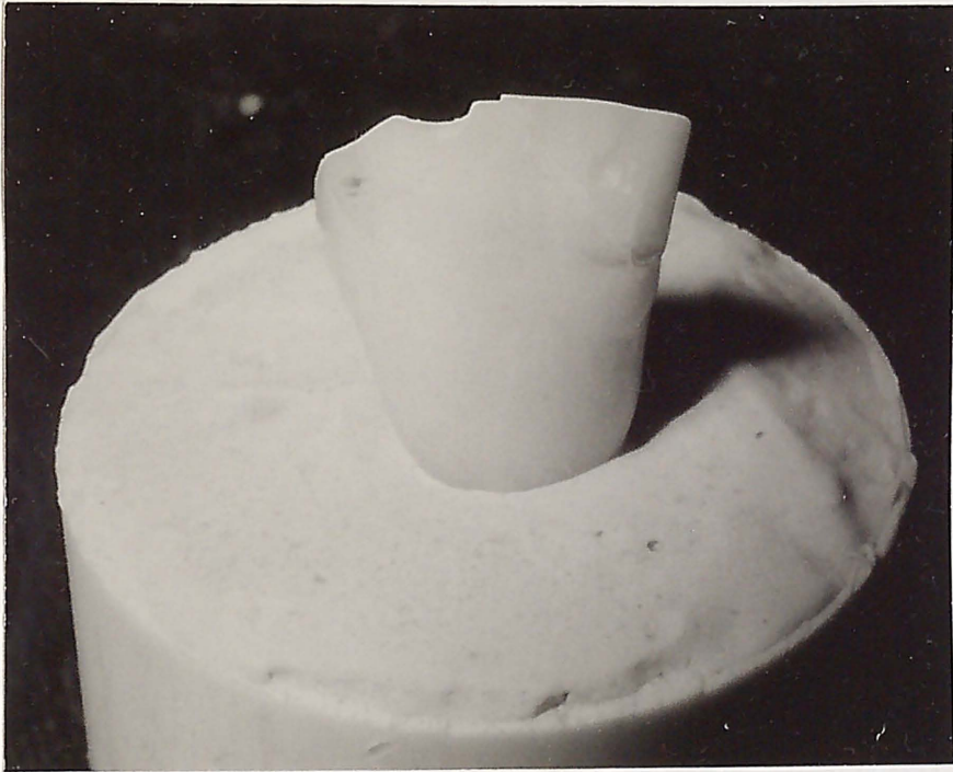
FIGURE 3. Mounted tooth showing dimple mark 1mm perpendicular to the fracture line.
