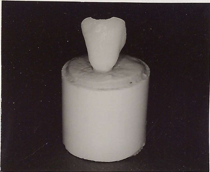
FIGURE 1. Bovine tooth mounted in acrylic ring with stone.
