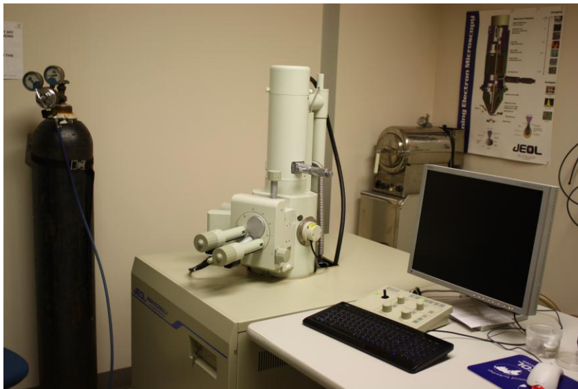
FIGURE 13. A JEOL SEM (JSM – 6390) used for surface micro-morphological evaluation
