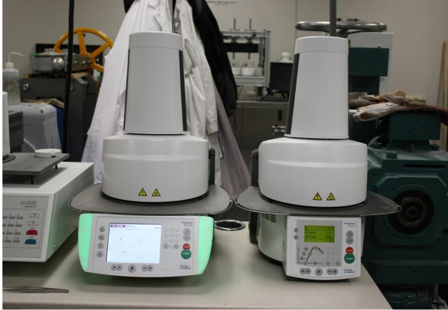
FIGURE 7. Furnace Programat EP 5000 (Ivoclar-Vivadent) used for ceramic processing
