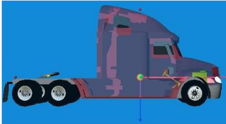
(a) Geometric profile of Volvo: The circle near the center of the vehicle indicates the center of gravity
