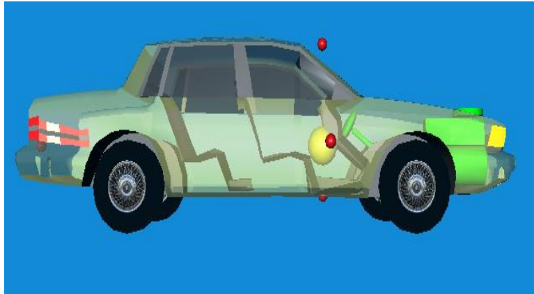
(a) Geometric profile of the Buick: The circle near the center of the vehicle indicates the center of gravity
