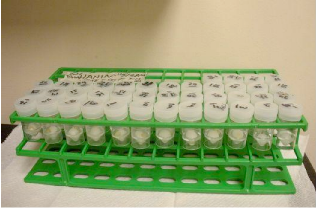
FIGURE 4. Specimens stored in separately marked vials with damp cotton pellets to preserve humidity.
