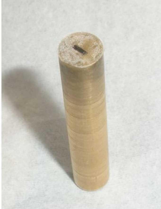
FIGURE 5. Holder with sample position marked for CT scanning of samples.
