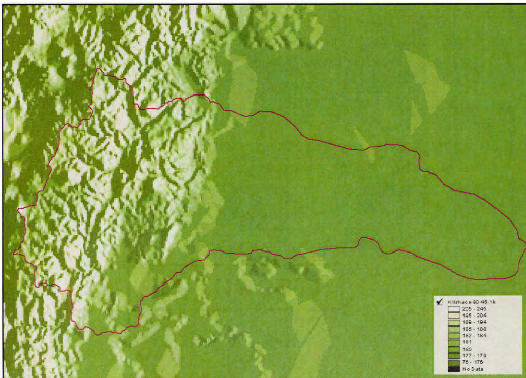
Figure H.4: Hill-shade map at 90° azimuth and 45° sun elevation for 1km resolution.
