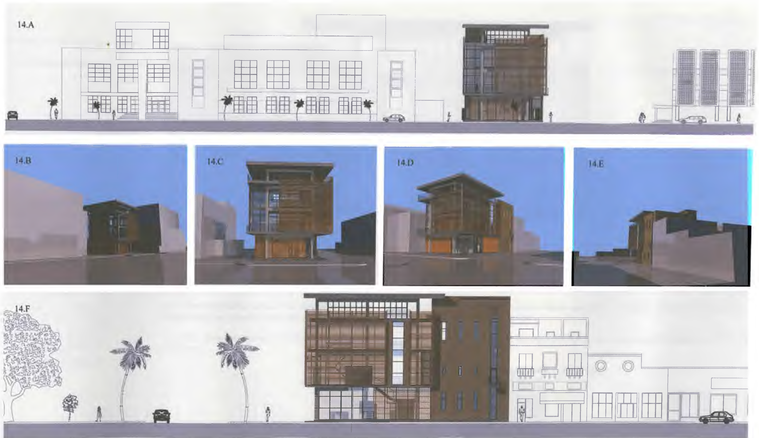
Figures 14.A - F: Massing studies. As the form of the project developed, its relationships to the surrounding buildings were analyzed. Figure 14.A is an elevation from the park looking north, showing how the project maintains a generally consistent height with the public library on the left and the hotel parking garage to the right. Figures 14.B through 14.E are a series of 3-d images created to study the form in context from the pedestrian level. Figure 14.F is an elevation drawing from Collins Avenue facing West, showing how the building serves to anchor its corner position while maintaining the upward stepping of the block to the South.
