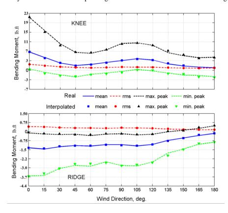
Figure 6.1 Interpolation between Models with Different Eave Heights
