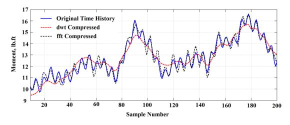
Figure 7.5 Comparison of Moment Evaluated Using Original Time Series and Compressed Data
