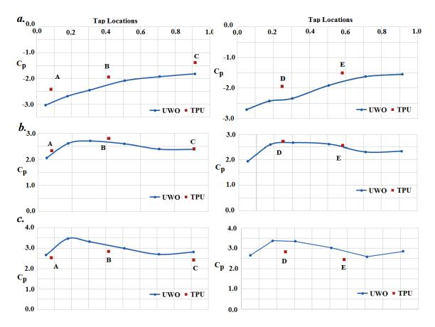
Figure 6.13 Expectation of Peak Pressure Coefficients (*Case 1-2*), a. 0 deg, b. 45 deg and c. 90 deg, wall.
