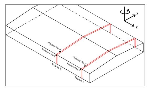
Figure 4.5 Location of Frames, and Taps for Pressure on Claddings
