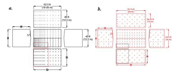
Figure 6.6 Exploded View: Buildings with Taps (Case 1-1), a. NIST and b. TPU.
