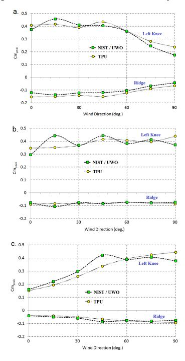
Figure 6.15 Peak Moment Coefficients, a. Frame 1, b. Frame 2 and c. Frame 3
