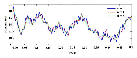
Figure 7.7 Example of frame response valuated using 500 Hz sampling rate (m=1) vs. obtained from data with reduced sampling rate (m=4, and m=8)
