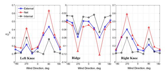
Figure 5.15 Peak External, Internal and Net Moment Coefficients, WOW model, Frame 3
