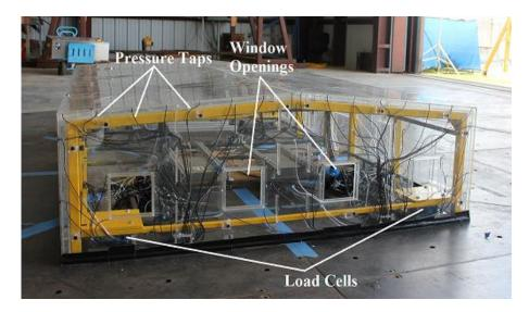
Figure 5.2. Wall of Wind Test Model
