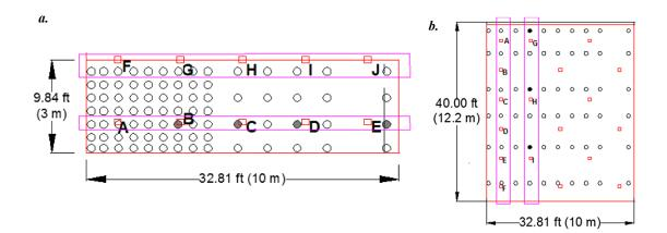
Figure 6.7 Details of Pressure Taps Selected for Comparison (*Case 1-1*), a. Roof and b. Wall.
