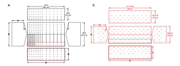
Figure 6.10 Exploded View: Buildings with Taps (Case 1-2), a. NIST and b. TPU.
