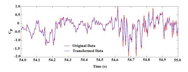
Figure 7.10 Example of original record (solid line) vs. record obtained from it by movingaveraged operation (dotted line).
