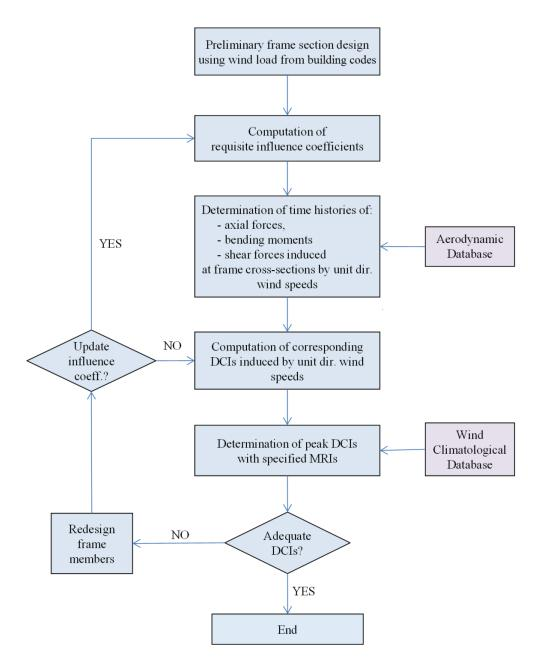
Figure 3.1 Overview of Design Procedure
