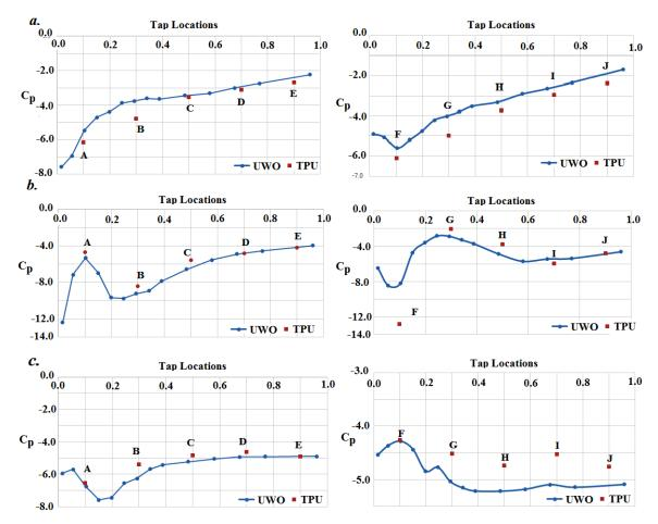
Figure 6.8 Expectation of Peak Pressure Coefficients (*Case 1-1*), a. 0 deg, b. 45 deg and c. 90 deg, roof.
