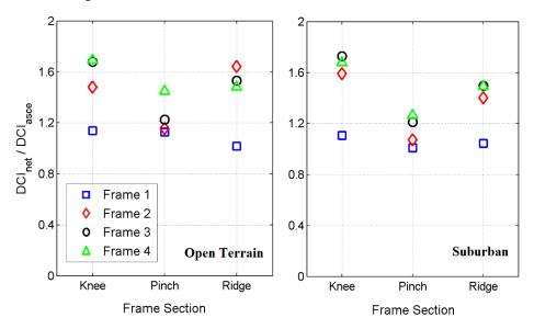
Figure 5.19 DCI<sub>net</sub> / DCI<sub>asce</sub> versus wind directions, NIST model 1
