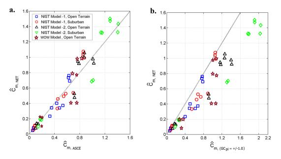
Figure 5.13 Experimental Computed  $\hat{C}_m$  versus  $\hat{C}_{m ASCE}$  and  $\hat{C}_{m (GCpi = \pm 1.0)}$
