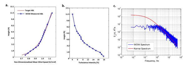
Figure 2.3 Simulation of open terrain ABL in the WOW: a) mean wind speed profile, b) turbulence intensity profile, and c) turbulence spectrum
