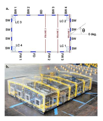
Figure 5.3. Large-Scale Model used in Experimental Investigation: Layout (upper) and Actual Model (lower)
