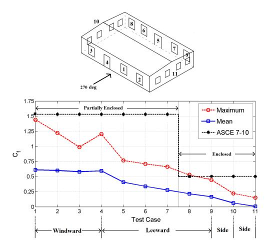
Figure 5.6. Mean and Maximum Roof Uplift Force Coefficients, Cfz
