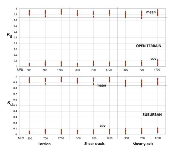
Figure 4.10 K<sub>d</sub>, Global Torsion and Shear, Hurricane Prone Regions
