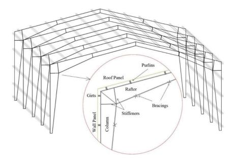
Figure 3.2 Layout of Addressed Structural System
