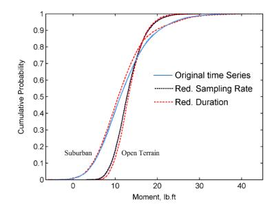
Figure 7.8 Comparisons of CDF of original time series to compressed time series 7.2.2.3. Refinement of the Sampling Rate Reduction Method
