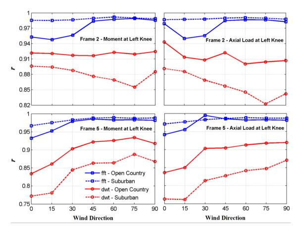
Figure 7.6 Comparison of  $r_M$  and  $r_P$  Evaluated at 90% Compression using *fft* and *dwt* Methods
