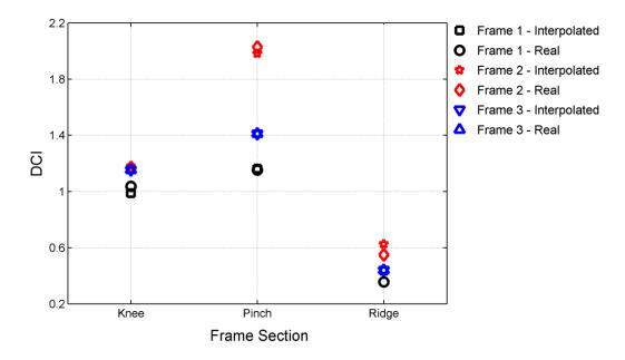
Figure 6.4 DCI<sup>PM</sup>s Based on Scaled Model of Building and on Interpolations from Models with Different Roof Slopes.
