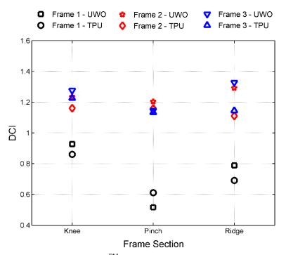
Figure 6.16 Comparison of DCIPM s Calculated using NIST and TPU Databases
