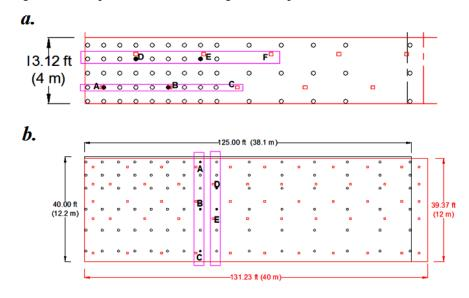
Figure 6.11 Details of Pressure Taps Selected for Comparison (*Case 1-2*), a. Roof and b. Wall
