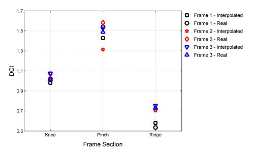
Figure 6.3 DCI<sup>PM</sup>s Based on Model of Building and on Interpolations From Models with Different Eave Heights.
