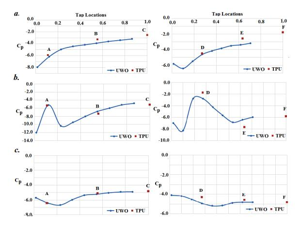
Figure 6.12 Expectation of Peak Pressure Coefficients (*Case 1-2*), a. 0 deg, b. 45 deg and c. 90 deg, roof.
