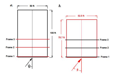
Figure 6.14 Plan View and Frame Layout of a. NIST and b. TPU Models Considered in Comparison
