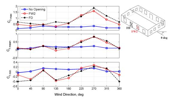
Figure 5.4. Mean and Maximum Roof Uplift Force Coefficients, C<sub>fz</sub>, Single Opening
