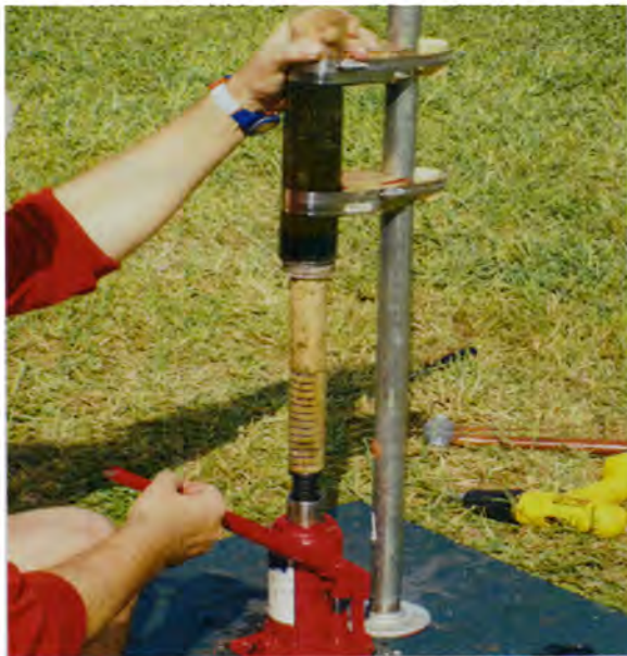
FIGURE 8 Sediment removal system. Hydraulic jack raises measured wooden dowels and rubber plunger through core barrel, pushing sediment up and out of the top.
